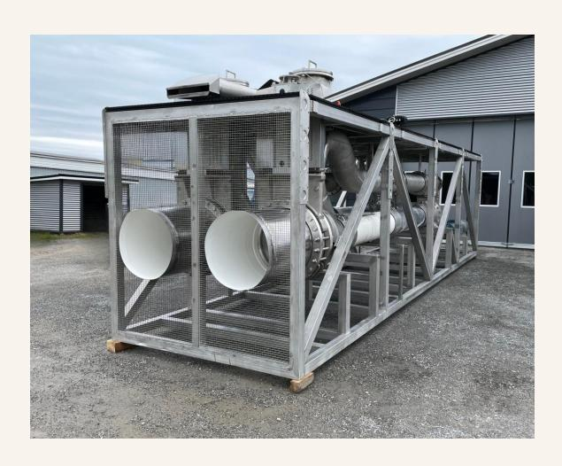
A floating unit, which has 2 fishway entries of which at least one is always open.
